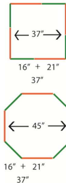
By doing this we accomplish two things. First, we are leaving the bag a size that fits well in trucks and overseas containers. We are also limiting the amount of the bag that can hang over the bottom by creating a large base. This is achieved by more efficiently using the perimeter of the bottom.
